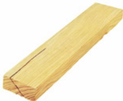
Splits are similar to checks except separations of the wood extend completely through a piece, usually at the ends.
