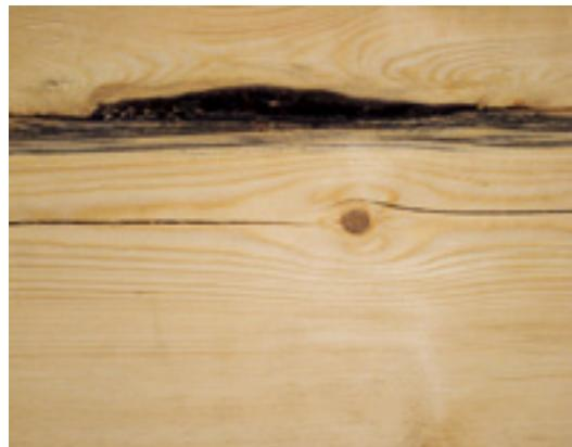
Heartstain — The first sign of a type of decay - referred to as incipient decay. Indicates that some wood strength reduction may have occurred. In structural lumber grades it is only restricted in Select Structural, the top grade in SLF and J&P. Many appearance grades do not limit heartstain as they do any other stain due to visual impact. Not in Chinese standards.
