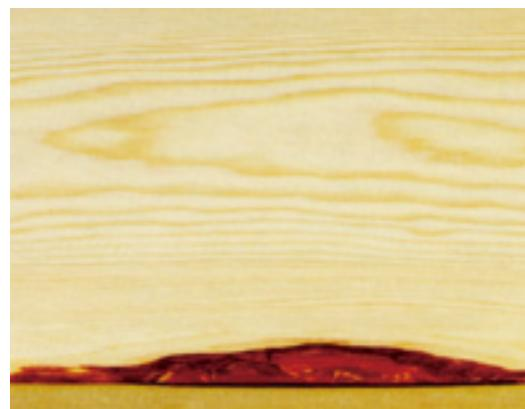
**Slope of Grain** — The term used to describe the angle of the wood fiber orientation. In most lumber the grain runs parallel with the edges, and therefore there is no slope of grain. When the grain runs off at an angle, strength and appearance is greatly reduced. Structural and appearance grades severely limit slope of grain for this reason. Slope of grain is not a common occurrence, and usually very few pieces of lumber from a mill run will be affected by it.
