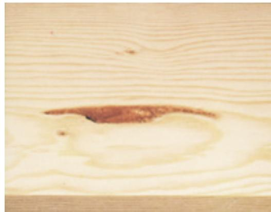
Bark Pockets — Formed when outer bark is grown over by the tree. Bark pockets are not restricted in structural lumber grades, but must be assessed as an equivalent characteristic such as wane, if they become excessive in size, or are located on the edge of a piece. These are very restricted in appearance grades of lumber, similar to knots.
