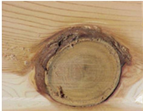
Fixed knot — An enclosed knot which will not move, due to its growth, shape, or position. It is often the irregular shape of these knots which keep them "locked" into place. Not restricted in any structural lumber grades, and treated the same as intergrown knots in most other graderules. Not in Chinds standards.
