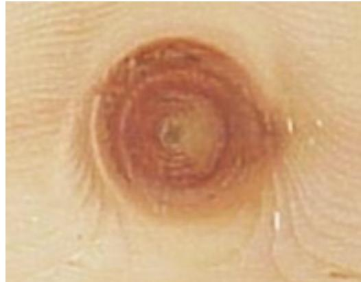
Oval knot — Simply refers to the knot shape, as a result of the tree branch being sawn thru at an angle between 0 and 90 degrees. Oval knots are still measured between lines parallel to lumber edges in structural lumber. For other grades of lumber, they are measured as an average of the length and width of the knot.
