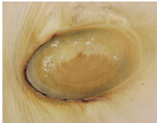
Spike knots — Found in vertical grain lumber, as a result of a tree branch being sawn along its axis. The size of spike knot is determined by mathematical formulas, which convert the spike knot shape to the equivalent round knot size. Large spike knots result in significant strength reduction due to their large displacement of wood fibre. Structural lumber is sawn flat grain to avoid spike knots.
