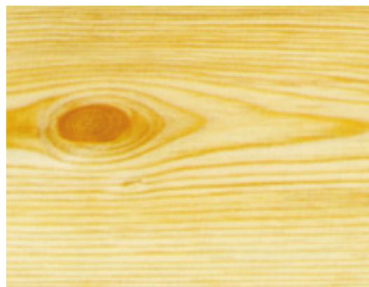
Enclosed knots — Knots which are NOT intergrown, and as a result have a layer of bark or pitch separating them from the surrounding wood. Such knots are less desirable because they may become loose and fall out. Not restricted in any structural grades, as long as the knot is still tightly fixed (won't move). Not in Chinds standards.
