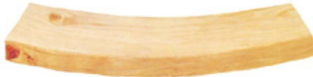
Crook is a deviation from a flat plane of the narrow face of a piece of lumber from end to end.
