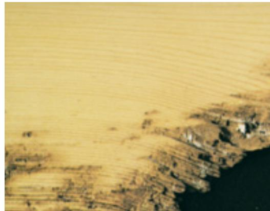
Pek — Is a type of decay that is only found in Cedar species. Although wood affected by pek has lost all structural integrity (can be crumbled under finger-nails), it will not spread further once the tree is cut. There is very little tolerance for this type of decay in most structural and appearance grades. It is treated as similarly to firm honeycomb - not restricted as tightly as unsound wood but more restricted than Whitespeck. Not in Chinds standards.
