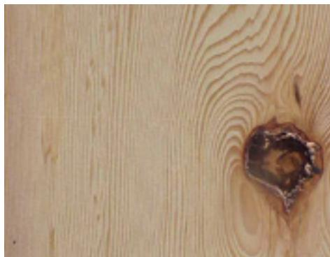
Unsound knot — Knots which contain decay. These knots are much less desirable and are restricted more than sound knots in Structural and Appearance grades of lumber.
