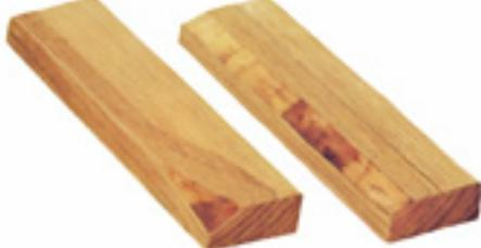
Wane is the presence of bark or lack of wood from any cause on the edge or corner of a piece of lumber.
